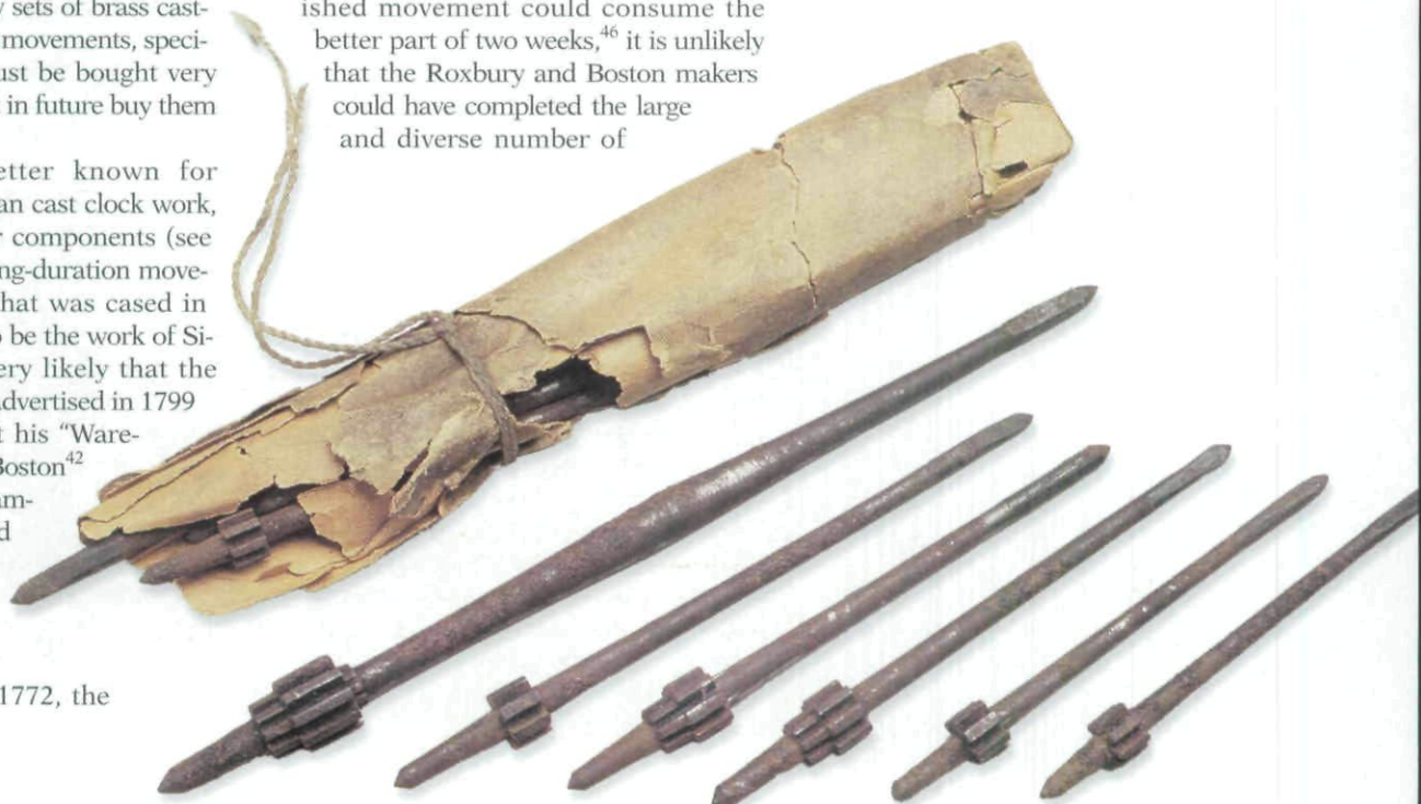
Pl. X. Nineteenth-century pinion set for an eight-day clock. Seven were required for each clock. Sets of slit pinions were sold in large numbers to suppliers throughout the United States. American Clock and Watch Museum; Arnold photograph.
